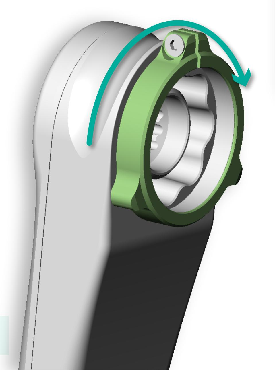
On left crank tighten the nut until it contacts the crank.
