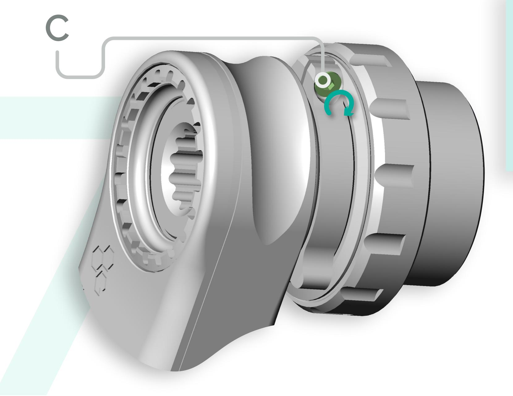
Tighten the securing bolt (C) on the preload adjuster by using a 2mm HEX key. Recommended tightening torque: 1-1.5Nm.
