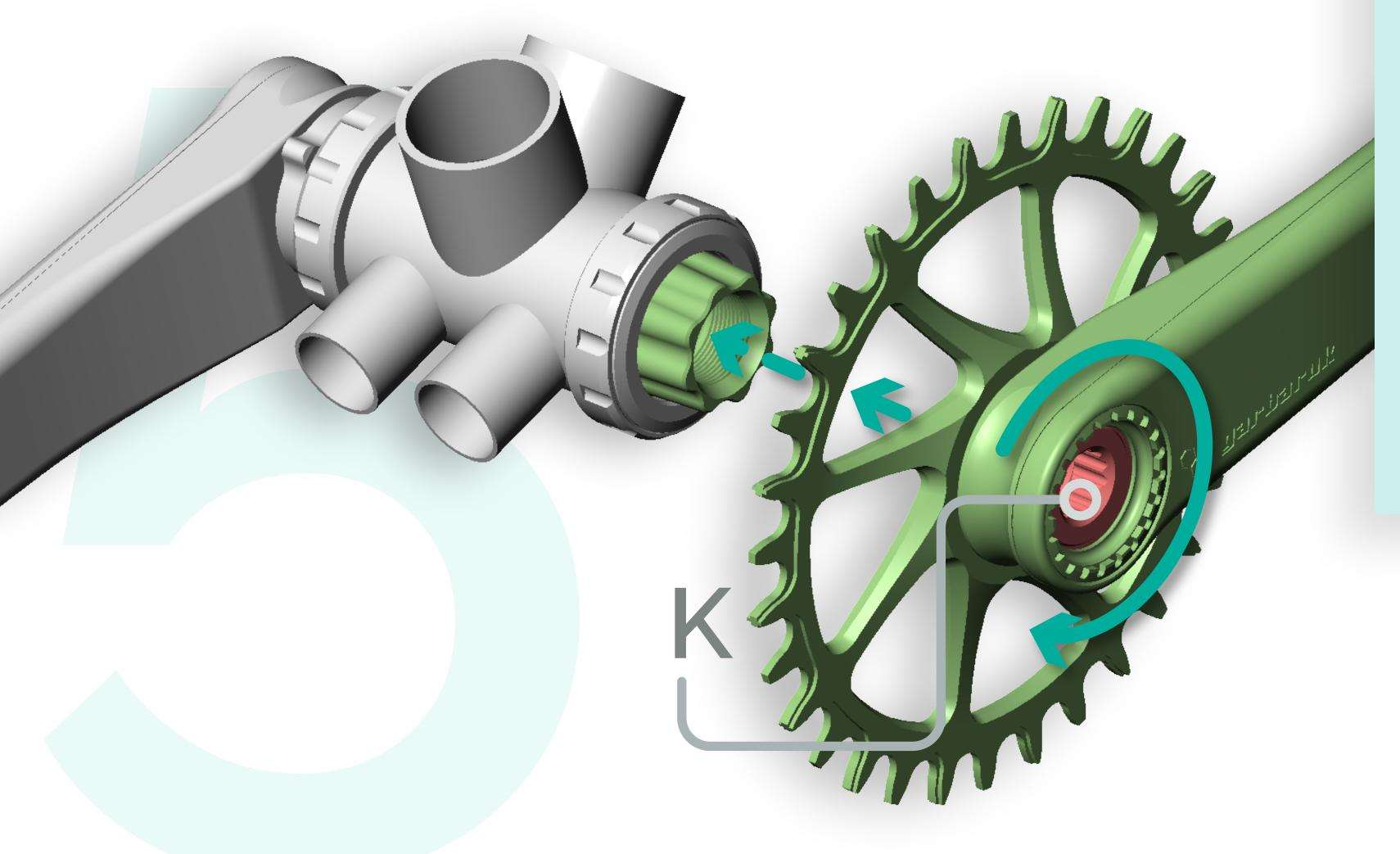
Mount the driveside crankarm. Secure by tightening the crankset bolt (K) with a 12mm HEX key.
