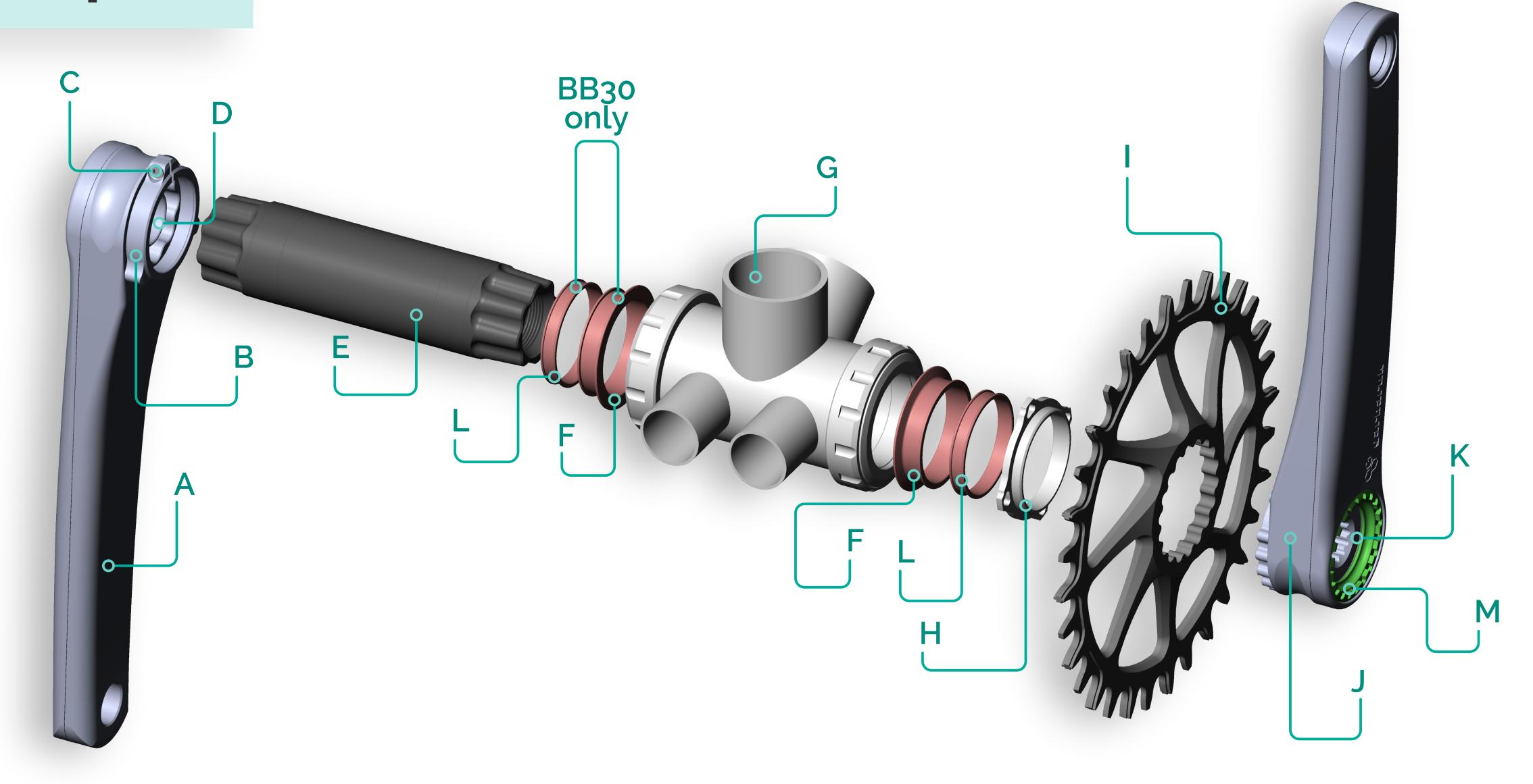
On the non-driveside crankarm, turn the preload adjuster (B) until it gently touches the crankarm (A).
